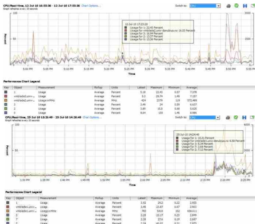
Figure 4 Monitoring resources load (CPU) Blade servers (1 and 2)
