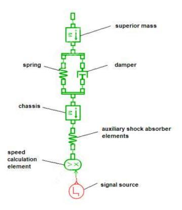
Figure 1. Simple Linear Mechanical Suspension Diagram
