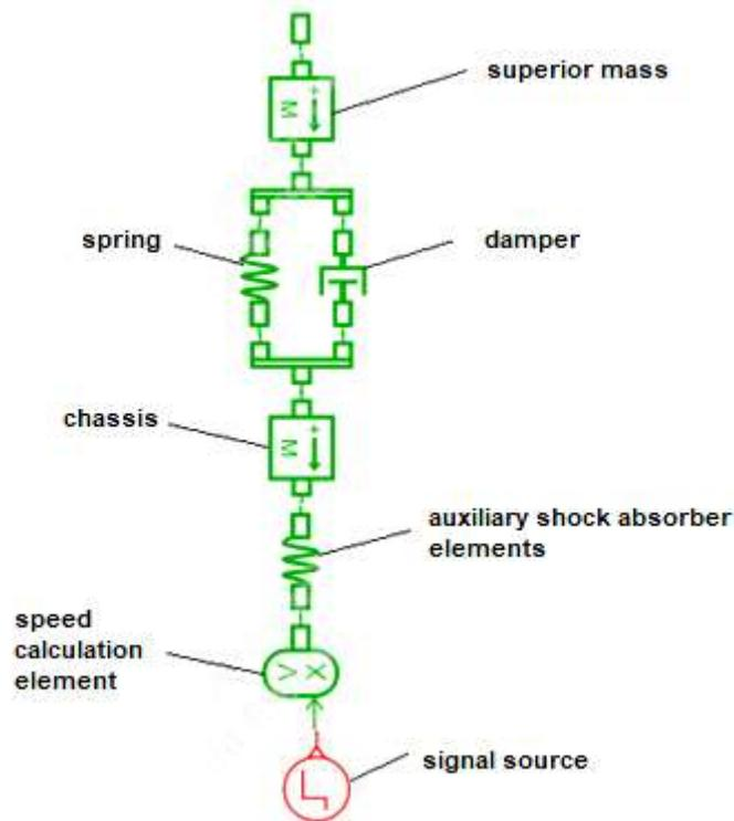
**Figure 1. Simple Linear Mechanical Suspension Diagram**
