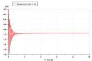
**Figure 4.** Movement of the Spring Mass Over Time
